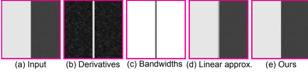
Fig. 4. Given a noisy step function (a), estimated derivatives (b) and bandwidths (c) computed for image position x are visualized. In this example, we do not use any geometries. While the linear approximation (d) with a large global bandwidth produces over-blurred results, our method (e) guided by the estimated bandwidths (c) preserves the strong edge.
