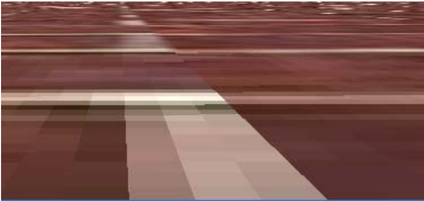
Mag. filter: nearest Min. filter: linear
