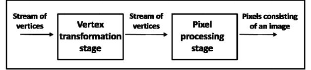
Since these two stages can be performed independently, we can perform these two stages in a parallel manner in graphics hardware. For example, after performing vertex transformation to v1, v2, v3, we perform rasterization step for a triangle consisting of those three vertices. During rasterizing the triangle, we can perform vertex transformation to other vertices, say, v4.
