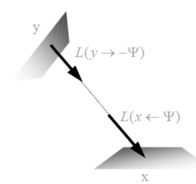
Ray-casting function: what is the nearest visible surface point seen from x in direction  $\Psi$ ?
