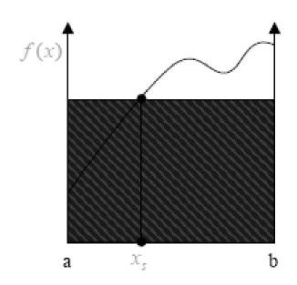
$$E(I_{prim}) = \int_{a}^{b} f(x)(b-a)p(x)dx = \int_{a}^{b} f(x)(b-a)\frac{1}{(b-a)}dx = I$$
