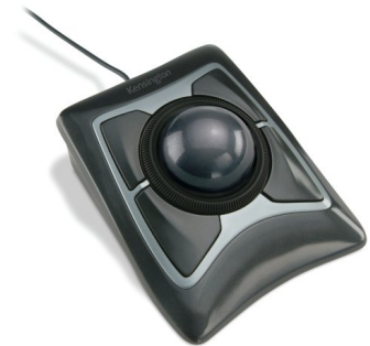
Figure 5.2: A trackball. The image is excerpted from the homepage of its vendor, Kensington.
